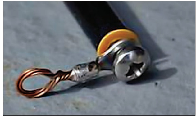
Fig. 6: Steve made up tie-point rings to be put into the ends of each spreader, making tying off easier.
