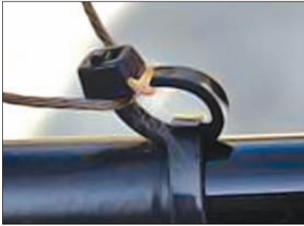
Fig. 7: Two 'tie-wraps make a good 'P'-clip, A few layers of insulated tape wrapped around the spreader. keep it from moving.
